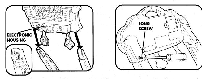
3. Turn assembly right side up. Slide electronic housing onto arms. Secure housing to arms using 2 long screws and Phillips screwdriver.
