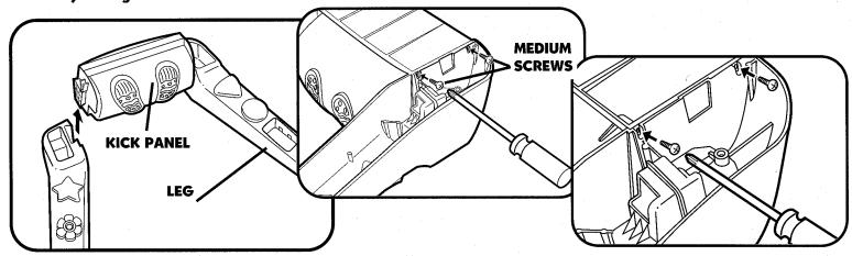
I. Attach kick panel to legs. Turn assembly upside down and place on flat surface. Using 4 medium screws and Phillips screwdriver, secure kick panel to legs.
