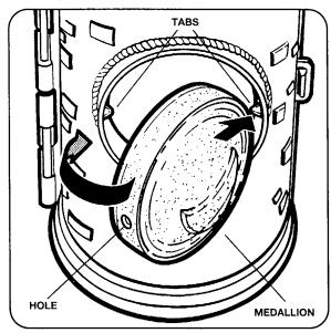
Align hole on one side of medallion with tab on one side of opening. Press other side of medallion into opening until tab snaps into hole.
