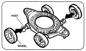
Position decorated side of wheels away from carriage bases. Slip wheels onto posts until wheels snap into place.
