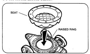
Press bottom of seat over raised ring on top of carriage base.
