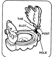
3. Align post and tab on right side of swing with hole and slot in swing seat, then press side into seat. Repeat for left side.
