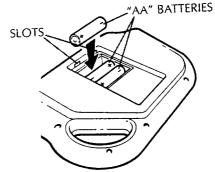
2. Remove exhausted batteries. Insert 3 fresh "AA" batteries as shown. Insert tabs on end of door into slots in compartment opening, and lower door into place. Tighten screw. Your computer is now ready to reboot!
