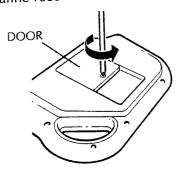
1. Using a Phillips screwdriver, loosen screw in battery compartment door on back of "computer terminal". (Screw will remain attached to door.) Remove door.
