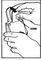
Fit cover into place as shown and snap shut. (Battery sold separately.)
