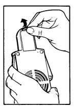
To remove battery cover, fit small coin into slot behind Major Morgan's head. Press toward center.
