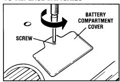
1. Loosen screw on battery compartment cover, and remove cover.
