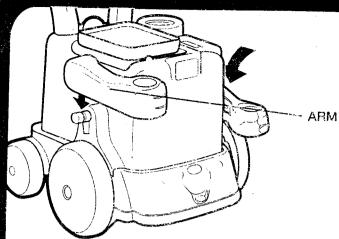
Snap arms onto posts on sides of cart. Make sure arms extend forward, as shown in illustration. (The arms are designed to pop off when meeting any resistance, such as if the cart runs into a wall. They easily re-attach to the posts.)
