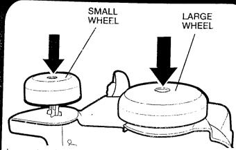
Lay cart on its side. Snap large wheels onto front wheel posts. Snap small wheels onto back wheel posts. Note: You have to press down very firmly when attaching the wheels, it helps to place your hand under the wheel attachment area and push up as you press down on the wheel.
