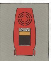
(2) Insert battery into compartment against correct contacts.
