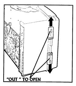
TO OPEN & CLOSE CASE: Slide latches "OUT" to unlock case. Slide latches "IN" to lock case.
