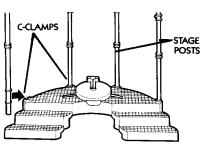
2. Snap four (4) stage posts into C-clamps on sides of stage. Make sure hollow sides of posts face rear of stage.
