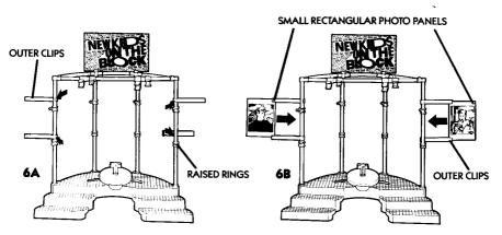
**6A.** Snap outer clips onto two (2) outer stage posts, above raised rings. Slots on lower clips should face up; slots on upper clips should face down.
