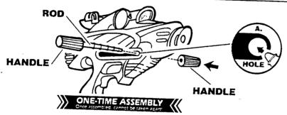
A. IMPORTANT: Carefully insert ROD all the way into the hole in the base unit so that the HANDLE touches the base unit.
