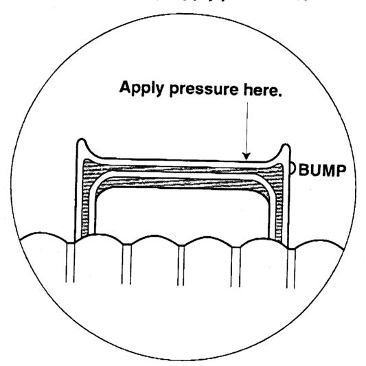
the side of the trigger with a bump as you squeeze the trigger halfway.
