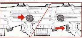
Pull Bolt Mechanism back. If Bolt Mechanism seems stuck, try pulling the trigger first.
