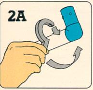
To unlock a tube from a connector, snap posts on Pipeworks "pipewrench" into holes in tube.
