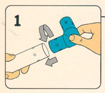
Slide the tube over the connector and rotate it until you hear it click into position. The locks on the connector should now be inside the holes in the tube. Always hold the back of each connector so you don't pinch your fingers between the tube and connector.
