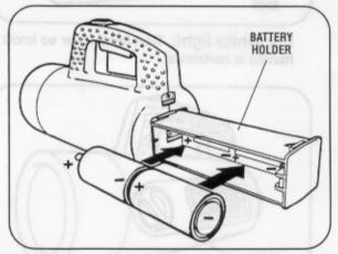
STEP 2. Slide out battery holder. Insert 2 "C" batteries as shown in diagram located inside battery holder.
