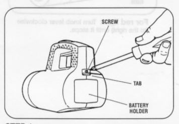
STEP 1. Locate tab on back end of flashlight. Loosen screw, located above tab, with a Phillips® screwdriver (not included). With thumbnail or coin, move tab up to unsnap battery holder.
