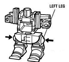
2. Now, assemble the Doh-Bot figure's left leg, once again sliding into place from the side, and locking the tabs on left leg into the slots on right leg as shown.
