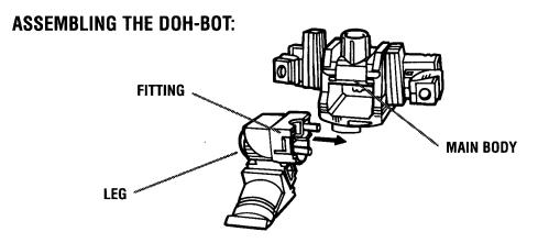
1. First, assemble the Doh-Bot figure's right leg, sliding the leg over the fitting underneath the Doh-Bot figure's main body piece from the side as shown.
