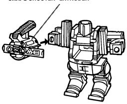
3. Snap the right arm "Shape Shooter" extruder into place. When assembled, the handle of the extruder should be on top as shown.
