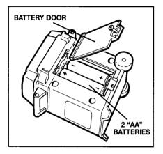
Locate battery compartment in back of barbecue grill. Use a Phillips screwdriver to loosen screw, and remove battery door. Insert 2 "AA" batteries (alkaline recommended) as shown, then replace door and tighten screw.
