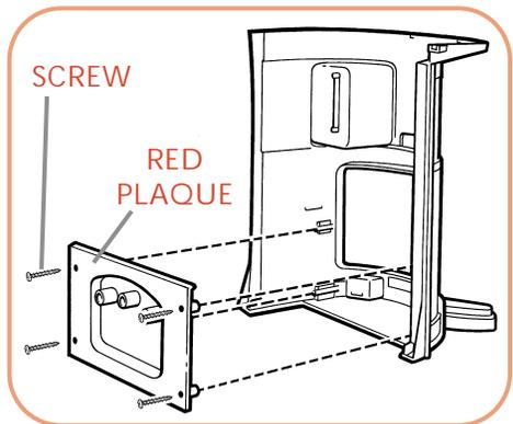
3. Attach and fasten the safe housing to the Playstore assembly. Fit safe housing inside fittings in Playstore, angling in the right side first, then the left. Secure housing to Playstore with 3 screws and the screwdriver.
