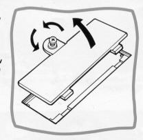
Insert 4 x 1.5V "AA" or LR6 batteries according to the diagram on the inside of the battery compartment.
