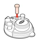
Position the launcher base on top of the metallic target, with the launcher post pointing up. Align the launcher base as shown with the grooves on the metallic
