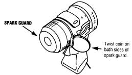
Use a coin to help slide spark guard up to reveal flint holes. Put edge of coin into position shown and twist so that spark guard slides up - first one side, then the other, until flint holes in spark quard are exposed. Do not remove spark guard.
