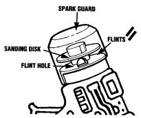
Hold welding gun as shown with spark guard pointing upward. Drop 2 flints into one of the holes on either side of the spark guard. Flints should be between the sanding disk and the front of the welding gun.
