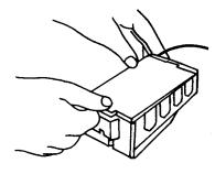
Replace lid by first inserting smaller tab of battery box lid into slot at wire end of battery box. Then snap lid closed.
