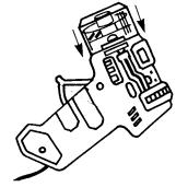
Push spark guard closed. IMPORTANT: Welding gun will not operate unless spark guard is fully closed. Flints are standard lighter flints. Do not use more than two flints in welding gun.
