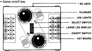
\* AC adaptor specifications: DC 9V at 500 mA load.
