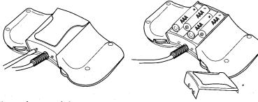
Unscrew the screws which are on the battery cover in the bottom part of the control pad.
