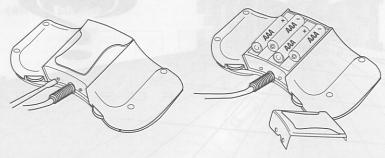
Unscrew the screws which are on the battery cover in the bottom part of the control pad. Insert 4 Alkaline "AAA" batteries, UM-4, LR03 or equivalent into the battery compartment. Close the compartment.
