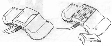
Unscrew the screws which are on the battery cover in the bottom part of the control pad. Insert 4 Alkaline "AAA" batteries, UM-4, LRO3 or equivalent into the battery compartment. Close the compartment.
