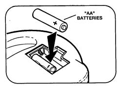
Remove and discard the batteries. Insert 2 new "AA" batteries (Eveready\* alkaline batteries are recommended for longer life). Replace the battery door and re-fasten the screw with the screwdriver.
