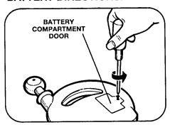
Rockin' Radio is equipped with 2 "AA" batteries. When they run out, use a Phillips® screwdriver (not included) to loosen the screw securing the battery compartment door and remove door. The screw remains attached to the battery door.
