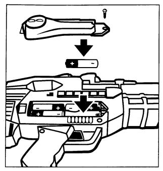
Remove worn batteries and insert fresh batteries. Replace cover and tighten screw.
