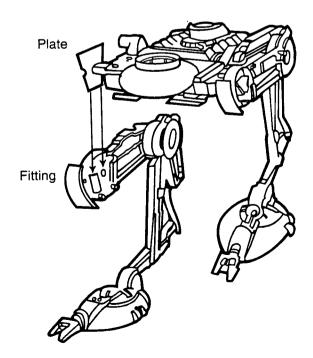
STEP 2: Make sure round hole in the link is placed over post.
