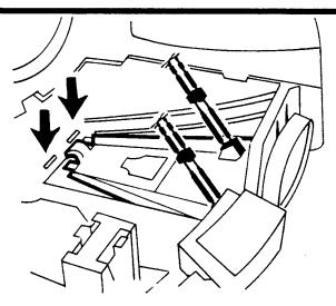
**10.** Snap the ramp onto the vehicle floor as shown. The ramp can be manually raised or lowered.
