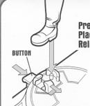
Press and hold button. Place foot in clamp. Release button.
