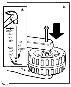
Fit push nut into push nut fastener tool. Position end of axle over push nut fastener. BE SURE TO USE THE LONGER AXLE FOR REAR WHEEL ASSEMBLY. LONGER AXLE IS SILVER. Using hammer, hit end of axle into push nut fastener. (See illustration a.)
