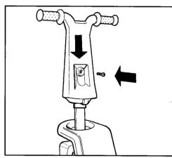
Slide handlebar onto fork **ALIGN THE HOLES** and attach with the 2 1/16"
