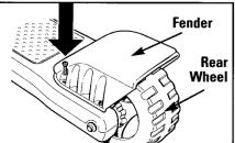
Fold the 2 clicker tabs inside the fender, and place fender over rear wheel as shown. Insert each 3/4" screw halfway in place, then go back and tighten all 4 screws firmly into position.
