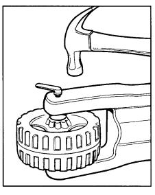
Turn body over. Fit push nut fastener into push nut fastener tool. Fit tool (with push nut fastener attached) over exposed end of axle. Using a hammer, hit fastener onto end of axle.
