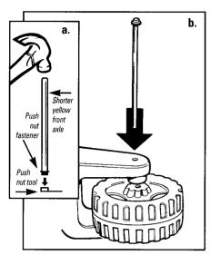
Fit push nut fastener into push nut fastener tool.
