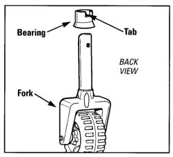
Place the bearing onto the fork, aligning the notches in bearing with fittings on fork. The tab on the bearing should face the back as shown.
