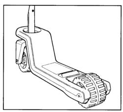
Slide fork through large opening in the front of scooter body as shown.
