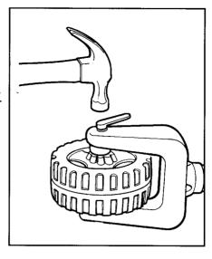
Turn fork over. Fit push nut fastener into push nut fastener tool. Fit too' (with push nut fastener attached) over exposed end of axle. Using a hammer, hit fastener onto end of axle.
