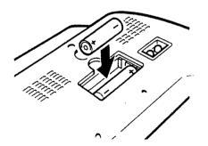
Insert 2 "AA" batteries into the compartment, following direction indicators inside compartment. Replace door and refasten with the screwdriver.
