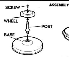
Remove screws that are attached to the bottom of the base. Push wide end of post into the top of the base. Fasten wheel to post with screw.
