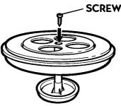
Flip assembly upsidedown, and push down on the base until the post touches the bottom of the base. Fasten post to the base of the screw.
