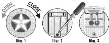
Remove the Battery-Speaker module by turning the star to the left. Pull out the module and turn it over. Open the battery compartment on the bottom of the module with a screwdriver. **See ilus. 1.2.3**.
