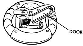
1. Using a Phillips screwdriver, loosen screw in battery compartment door on back of toy. (Screw will remain attached to door.) Remove door.
