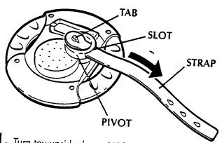
1. Turn toy upside down. With tab on strap facing up, slide strap through slot in pivot, from inside of pivot to outside, until round end of strap is in center of pivot.
