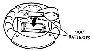
2. Remove exhausted batteries. Insert 2 fresh "AA" batteries as shown. Slide end of door under tab on compartment opening, and lower door into place. Tighten screw.
