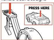
Push in latch on front of chassis to remove car body from chassis.
