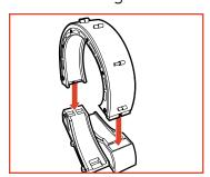
4. Fit lip on flexible track into top slot on base piece (garage side). Press down arrow on track and fully insert lip into base piece.
