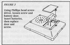
Insert the batteries into the coffin unit as shown in Figure 3. Be sure to match up the "+" and "-" symbols on the inside of the battery compartment.
