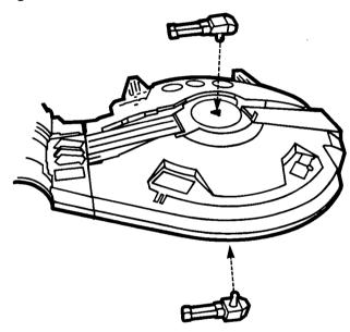
**4.** Attach the cockpit canopy. Slide the pegs on the vehicle, one at a time, into the holes in the hinge of the canopy.
