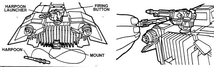
**4.** LASER CANNONS - Find the flat surface on the end of the laser cannons. Insert each laser cannon into place with the flat side down as shown.
