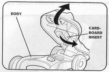
3. Attach Handle Assembly to Body Lift body and remove cardboard insert.
