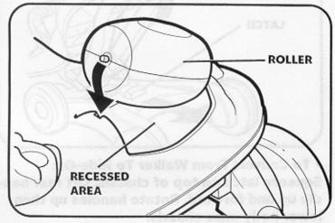
Turn body/chassis right side up and lower chassis onto body. Insert posts on roller into holes in recessed area (smaller post into smaller hole, larger post into larger hole).
