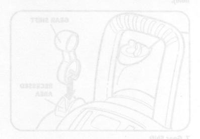
Gear shift fits only one way, inserts posts on goar skift into holes in recessed area (smaller post into smaller hole, larger post into larger hole).
