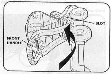
Turn body/chassis on its side. Insert front handle through slot in body.
