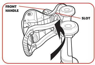
Turn body/chassis on its side. Insert front handle through slot in body.
