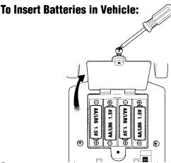
Remove screws on battery compartment door located on bottom of vehicle.
