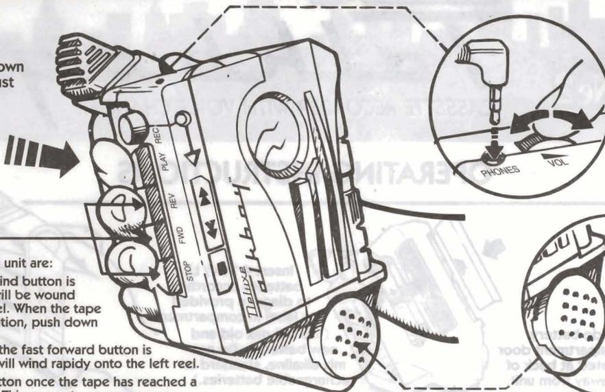
Near the microphone are the VOLUME control and the PHONES JACK. To increase or decrease the sound level during play back, rotate the wheel. To use headphones (not included) press into jack hole.
