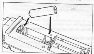
The + end of each battery must be inserted into the small, round, white plastic support, as shown
