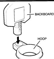
2. Insert BACKBOARD post fully into post hole on HOOP.
