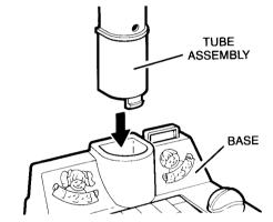
1. Insert TUBE ASSEMBLY into hole in BASE and push in until clips on TUBE ASSEMBLY snap into slots on bottom of BASE.
