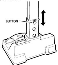
TO ADJUST THE HEIGHT OF THE HOOP Press the button on tube assembly and move the backboard/hoop assembly up or down, allowing the button to catch in one of the three holes.
