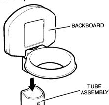
3. Insert BACKBOARD post into TUBE ASSEMBLY and push in until tabs on post snap into holes in tube.
