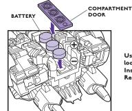
Using a Phillips/cross head screwdriver (not included), loosen screw in battery compartment door. Remove door. Insert 3 x 1.5V "A76" or LR44 size alkaline batteries. Replace door and tighten screw.
