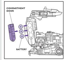
Using a Phillips/cross head screwdriver (not included), loosen screw in battery compartment door. Remove do Insert 3 x 1.5V "A76" or LR44 size alkaline batteries. eplace door and tighten screw. See diagram for polarity.
