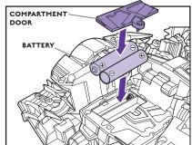
Using a Phillips/cross head screwdriver (not included), loosen screw in battery compartment door. Remove door. Insert 2 x 1.5V "AAA" or R03 size batteries. Alkaline batteries recommended. Replace door and tighten screw. See diagram for polarity.
