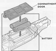
Using a Phillips/cross head screwdriver (not included), loosen screw in battery compartment door. Remove door. Insert 2 x 1.5V "AAA" or R03 size batteries. Alkaline batteries recommended. Replace door and tighten screw. See diagram for polarity.
